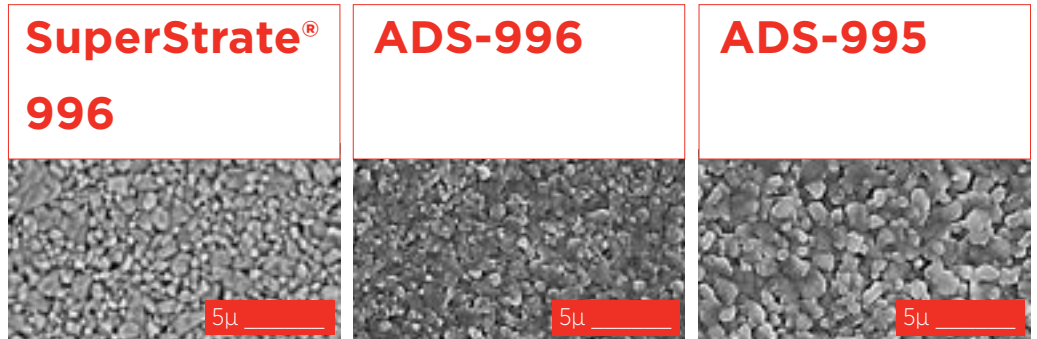
Figure 1. Scanning Electron Photomicrographs of "A" side (2,000x and 0° tilt).
